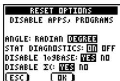
By default, the angle mode is set to DEGREE, Stat Diagnostics are ON, and the functions logBASE and summation ( $\Sigma$ ) are disabled.
