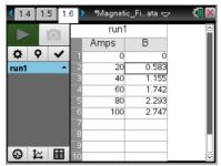
6. To complete the experiment, students are to increase the amperage in intervals of 20 mA up to 100 mA. For each voltage, they will click the Keep button to record the data. Note: The last column, magnetic constant will be calculated later.
