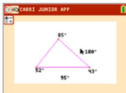
9. Press **clear** to stop the measurement tool and move the arrow to one of the three triangle vertices. The arrow will become "hollow" to indicate that the vertex being selected.
