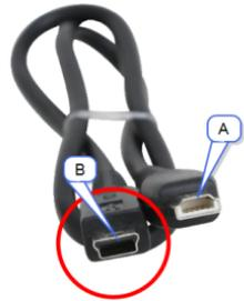
3. Insert the free end of the cable (the "A" connector) into the USB port on the calculator.
